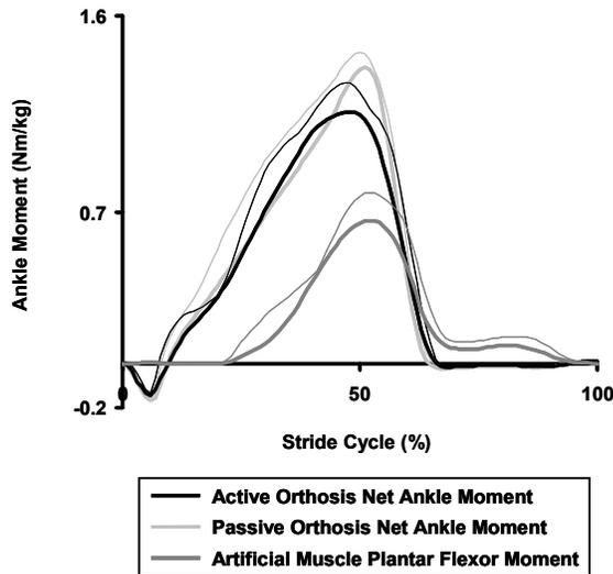
**Figure 2.** Mean + standard deviation of net ankle moments and artificial pneumatic muscle moments for the three subjects during overground walking at 1.0 m/s. Plantar flexion moments are in the positive direction. Subjects walked with very similar net ankle moments for the passive and active orthosis conditions when using foot-switch control.
